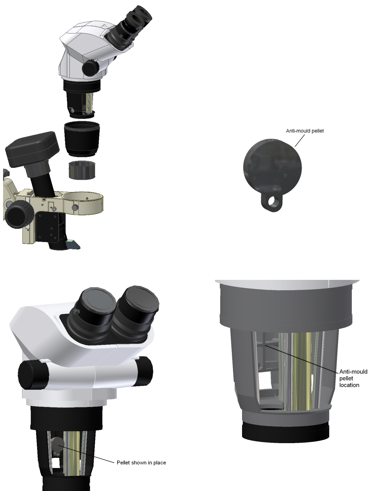
Figure 42, Fitting the Anti-mould pellet.
