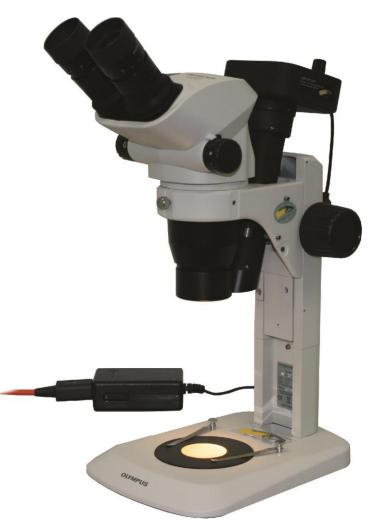
The SO-1700 LED gives excellent image quality and good depth of field over a continuous magnification range of 4.2x - 25x. The microscope is mounted on a sturdy base for wet laboratory use.
