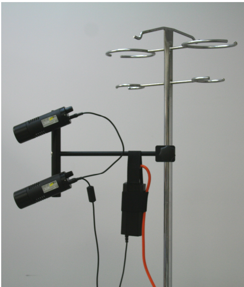
Figure 8 Assembled Surgical Lights attached to drip stand
